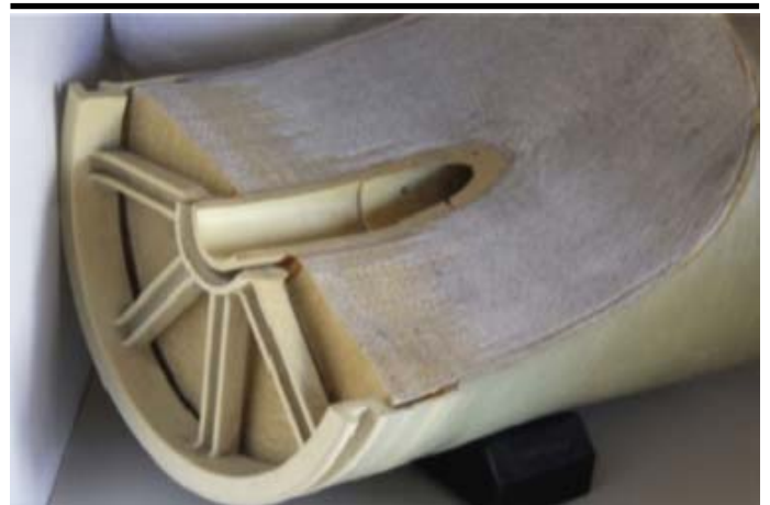
Cutaway of RO element showing spiral wound membranes
